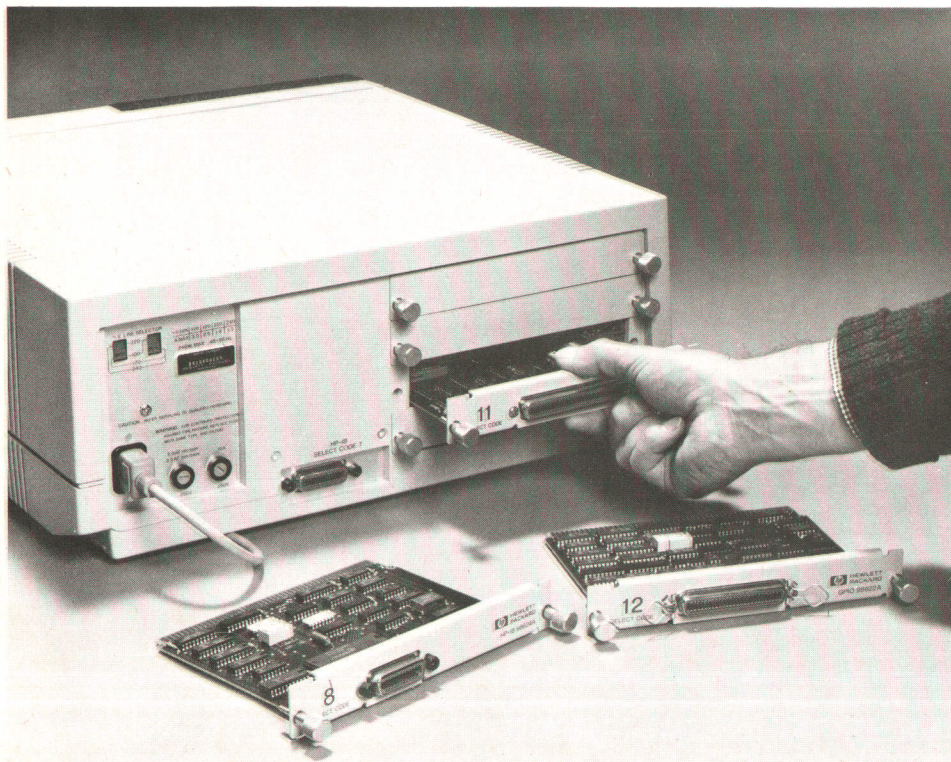
Fig. 3. The backplane of the 9826A and 9836A mainframes accommodates up to four I/O interfaces and four RAM, ROM, or DMA cards in addition to the internal HP-IB.
